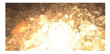
Code: DSGV Description: **Deposits Settled Gravel** Distance (ft): 7.3 Structural Grade: 0 O&M Grade: 2 Clock Start/From: 12 Clock To: 12 1st Value: 2nd Value: Value Percent: 10.000 Step: NO Remarks:
