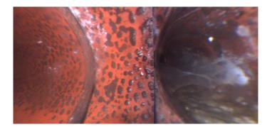
Distance (ft): 56.0 Structural Grade: 0 O&M Grade: 2 Clock Start/From: 3
