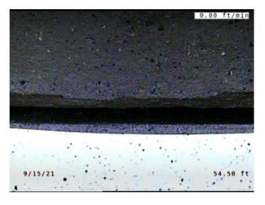
Code: MMC Description: **Miscellaneous Material Change** Distance (ft): 54.5 Structural Grade: 0 O&M Grade: 0 Clock Start/From: Clock To: 1st Value: 2nd Value: Value Percent: Continuous Index: Within 8" of Joint: NO Remarks: VCP TO PVC
