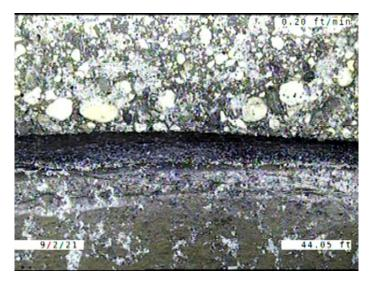
Code: MMC Description: **Miscellaneous Material Change** 44.0 Distance (ft): Structural Grade: 0 O&M Grade: 0 Clock Start/From: Clock To: 1st Value: 2nd Value: Value Percent: Continuous Index: Within 8" of Joint: NO Remarks: CONCRETE TO VCP
