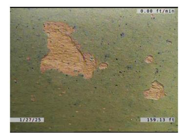
Code:SSCDescription:Surface Spalling of Damage Coating
