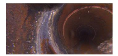
Distance (ft): 131.9 Structural Grade: 0 O&M Grade: 2 Clock Start/From: 7 Clock To: 10
